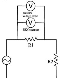
Figure 5- Measuring voltage across a resistor using a voltage divider
