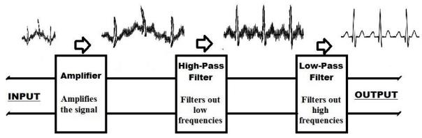
Figure 3 - Block diagram of EKG functions
