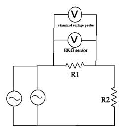
Figure 6- Circuit diagram using the LabQuest as two function generators, one to act as a 1 Hz "signal" and one to output the "noise".
